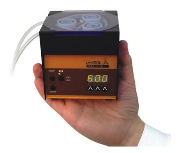
LAMBDA PRECIFLOW, MULTIFLOW, HIFLOW, MAXIFLOW and MEGAFLOW laboratory peristaltic pumps are specially designed for long term continuous processes with flow rates from 0.2 µl/min to 60'000 ml/hour. High precision, reproducible and long term stable flow rates are achieved with the quartz driven motor and unique tubing compression technique in the large pump head.
